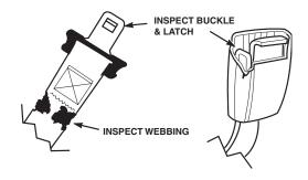
Figure 2-3. Seat Belt Inspection
